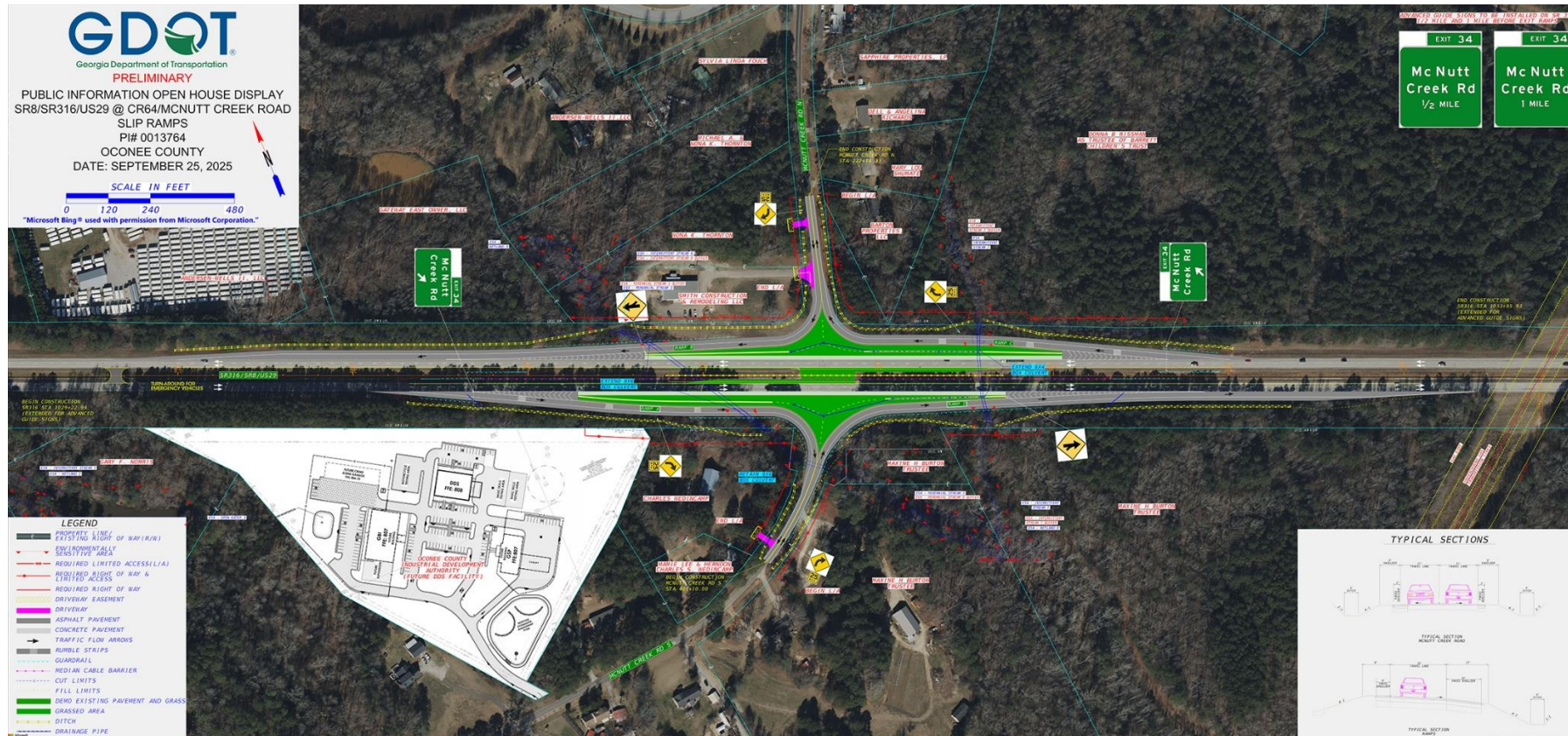
Proposed right-in, right-out slip ramp with a median break for emergency vehicles west of McNutt Creek Road
